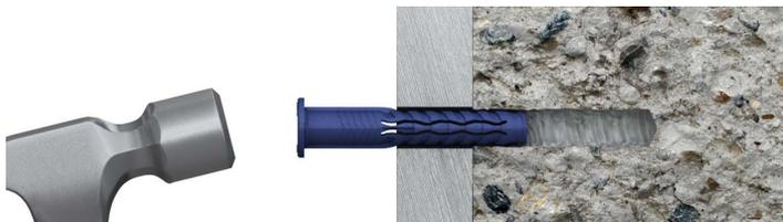
Step 4: Insert the screw and drive it home with the required tightening torque.
